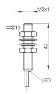
Inductive Sensors BES M08MG-USC20B-BV03 M 8 x1 x 40 normally-open Sn=2mm shielded
